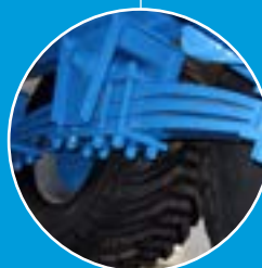
Pre-Tensioned Drawbar Suspension For smoother travelling
