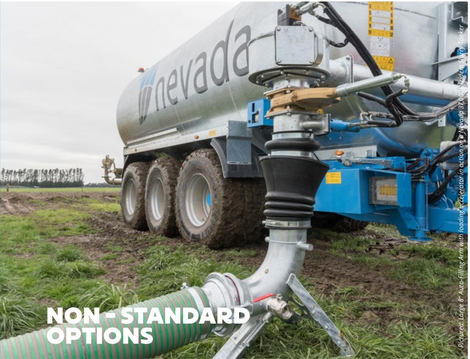
Pictured: Large 8" Auto-Filling Arm with loading accelerator in action on a Nevada 37,000L Tridem Slurry Tanker
